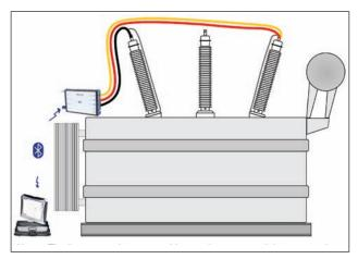
The laptop can be operated by touch screen and the communication is wireless via Bluetooth. Measurement ground braids connect close to the connection clamps and run next to the bushing to the flange connection to avoid cable loops that otherwise affect the measurement.
