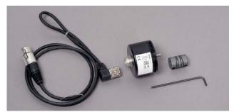
Rotary transducer, Novotechnic IP6501 (analog)
