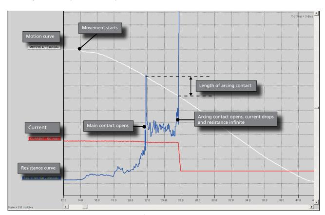
DRM is a reliable method to estimate the length/wear of the arcing contact. The SDRM202 provides high current and the TM1700 gives an accurate measurement with very good resolution. Besides, it is possible to use DualGround testing.
