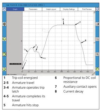
Example of coil current on circuit breaker
