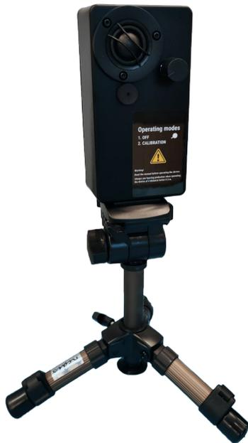
**NL Sonic Tester** is a reference sound source used to ensure the accuracy of the **NL Camera**.
