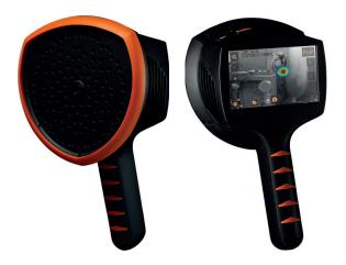
The NL Camera is an easy-to-use, stand-alone device for detecting and localizing partial discharges in medium and high voltage electrical systems during routine inspections. The NL Camera utilizes 124 microphones to find sounds emitted by partial discharges—even when they are completely inaudible to the human ear. Sound appears before components start to heat up, and the NL Camera enables detecting problems at an early stage.
